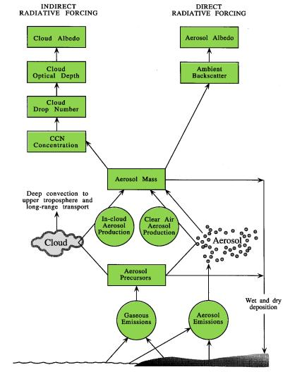
Figure 1. Direct and indirect mechanisms of aerosol effects on radiation and climate.
